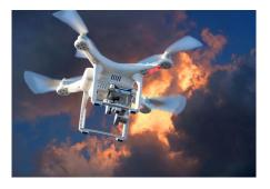
The QC government will benefit from these drones because they are equipped with different sensors mainly used in measuring rainfall amount, humidity, temperature, pressure, dew point, and other weather parameters that is essential on both weather forecasting and nowcasting
