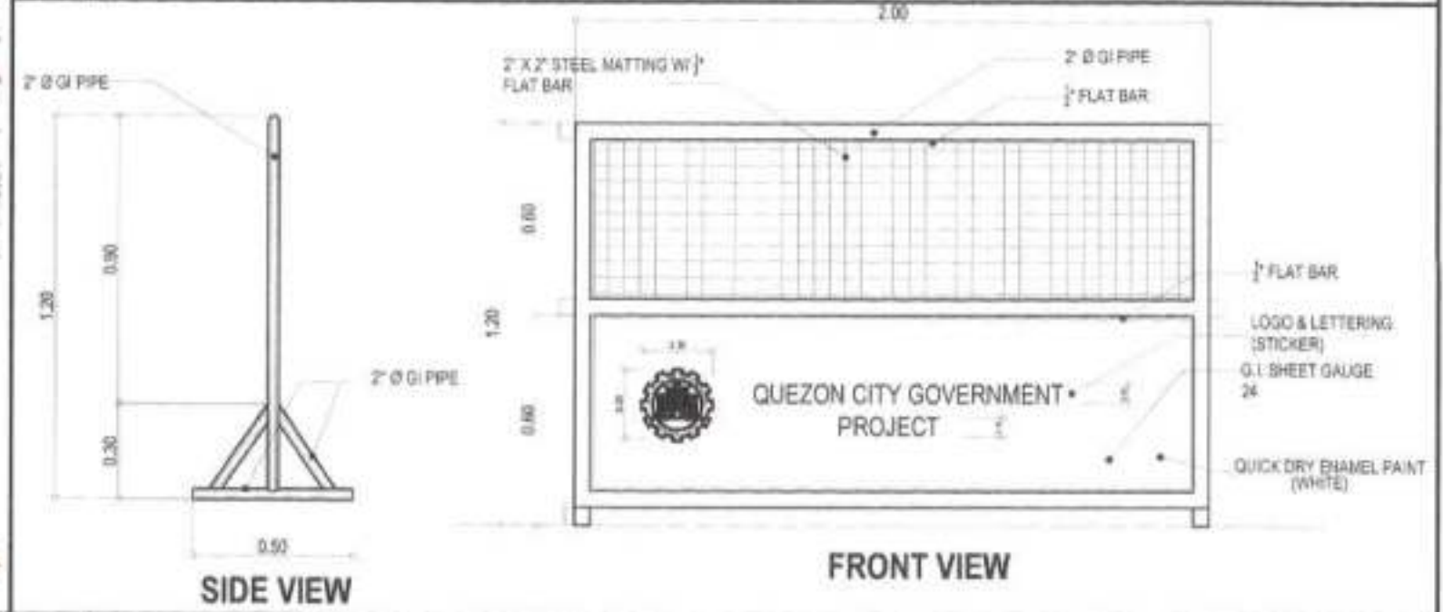
3 STEEL BARRICADE DETAIL
