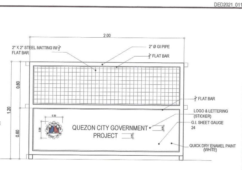
**4 STEEL BARRICADE DETAIL** SCALE : NTS
