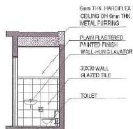
7 TYPICAL DETAIL OF COMFORT ROOM NTS
