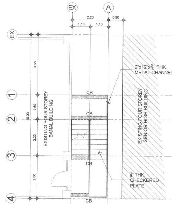
**1 GROUND FLOOR FRAMING PLAN EMERGENCY FIRE EXIT PLAN** SCALE:1:100m. **2 TYPICAL SECOND & THIRD FLOOR FRAMING PLAN EMERGENCY FIRE EXIT PLAN** SCALE:1:100m. **3 FOURTH FLOOR FRAMING PLAN EMERGENCY FIRE EXIT PLAN** SCALE:1:100m.
