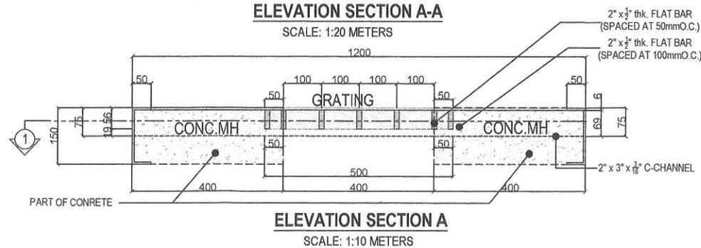
**1 PROPOSED MANHOLE DETAIL FOR 30"Ø RCP**
