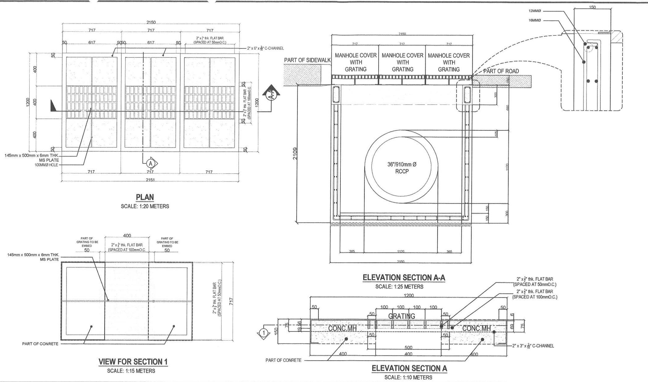
**1 PROPOSED MANHOLE DETAIL FOR 36"Ø RCP** SCALE : NOT TO SCALE
