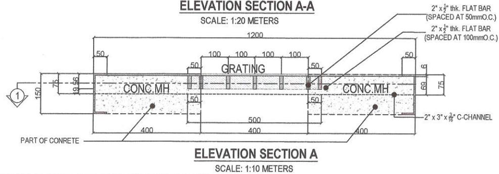
**1 PROPOSED MANHOLE DETAIL FOR 30"Ø**
