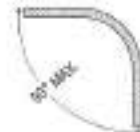
SINGLE ANGLE OF ANY BEND SHALL EXCEED 90°
