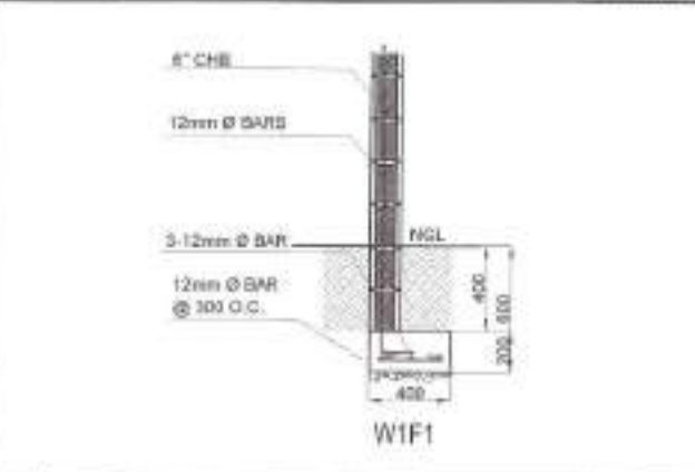
3 WALL FOOTING DETAILS SCALE 1:30M
