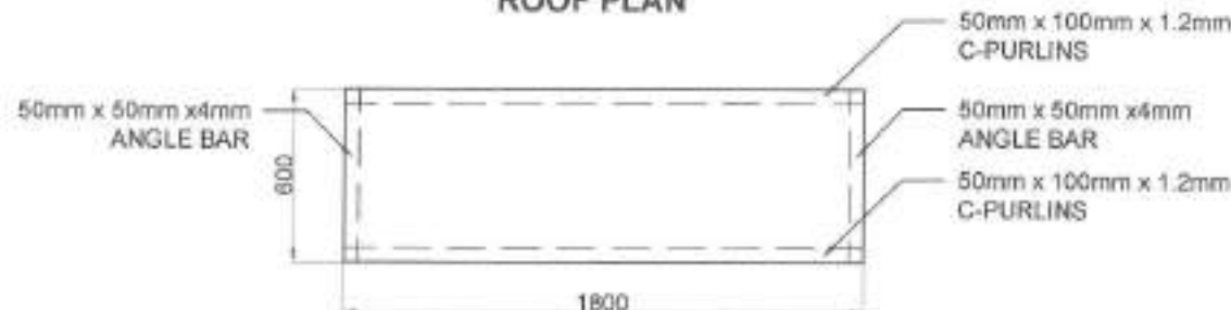
ROOF FRAMING PLAN
