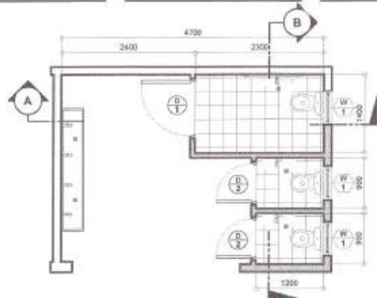
1 TOILET LAYOUT (DEPED COMFORT ROOM NEAR BELMONTE A)
