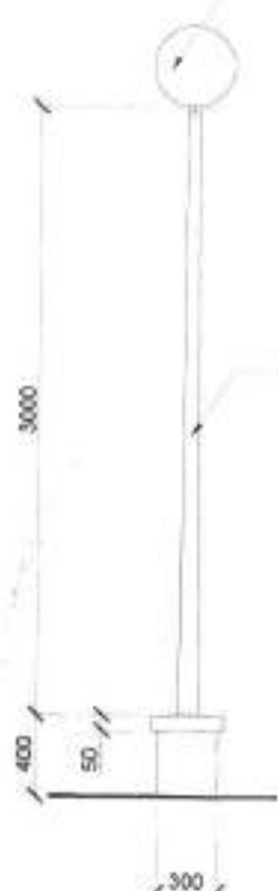
A PARK LAMP DETAIL SCALE 1: 30 MTS
