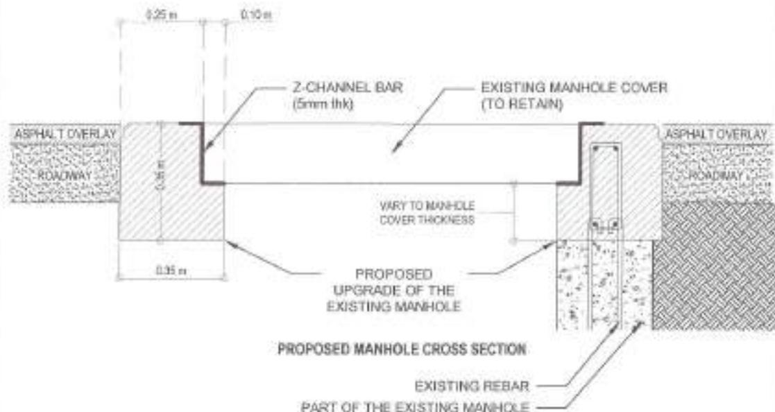
PROPOSED MANHOLE CROSS SECTION
