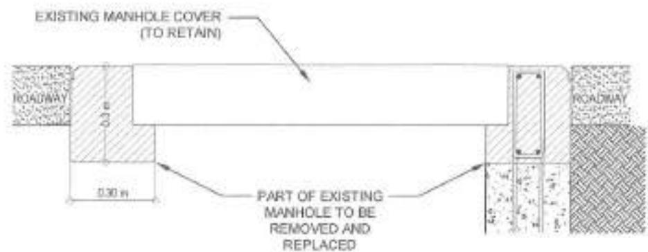
EXISTING MANHOLE CROSS SECTION
