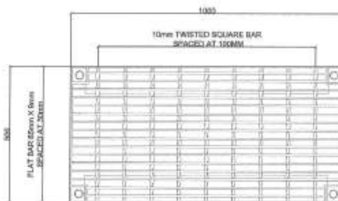
1000mm X 500mm STEEL GRATING MANHOLE SCALE: 1:10MTR
