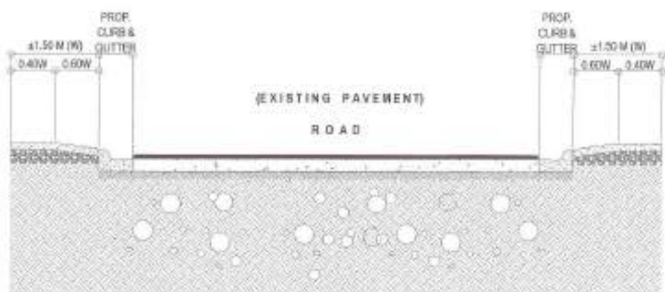
2 TYPICAL ROADWAY CROSS SECTION FOR REHABILITATION OF SIDEWALK (±1.50M) SCALE: NTS
