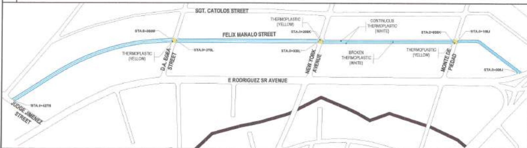
1 ROADWAY PLAN WITH THERMOPLASTIC LANE MARKINGS OF FELIX MANALO STREET
