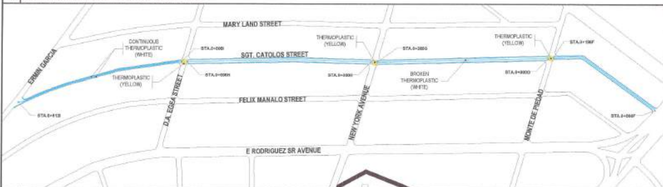
1 ROADWAY PLAN WITH THERMOPLASTIC LANE MARKINGS OF SGT. CATOLOS STREET
