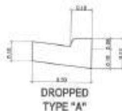
3 TYPICAL DROPPED CONCRETE CURB DETAIL
