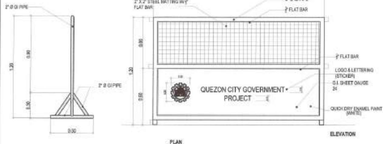
2 STEEL BARRICADE DETAIL
