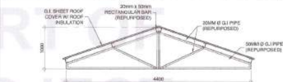
7 TRUSS DETAIL (B-4 SHED FOR LIVESTOCK)
