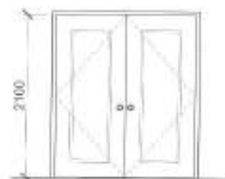
D-1 45mm THK POWDER COATED STEEL DOOR W/ COMPLETE ACCESSORIES SET 2 LOCATION: MAIN DOOR
