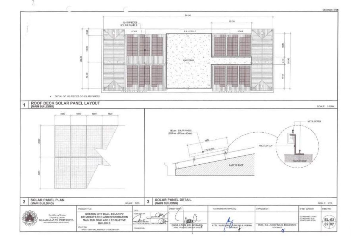
EXISTING PLUMBING VENTS, EXHAUST DUTLETS, VENTILATION INTAKE AIR OPENINGS SHALL NOT BE COVERED BY THE PHOTOVO-TAIC SYSTEM.
