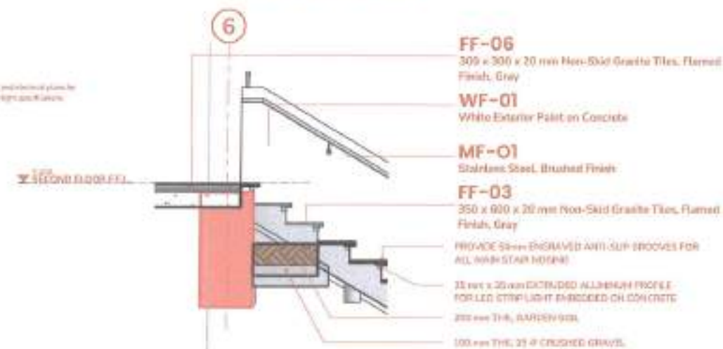
4| MAIN STAIRS SECTION BLOWUP 1
