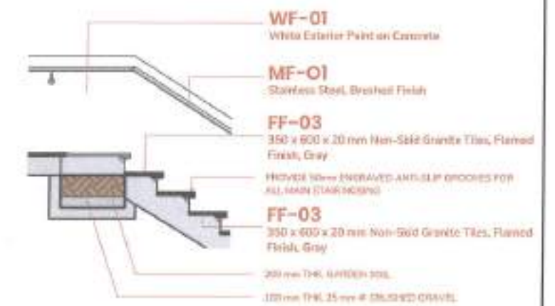
5| MAIN STAIRS SECTION BLOWUP 2
