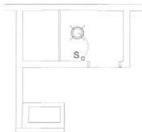
3 FINANCE ROOM TOILET LIGHTING LAYOUT (RIZAL BUILDING) SCALE: 1/4"=1'-0"
