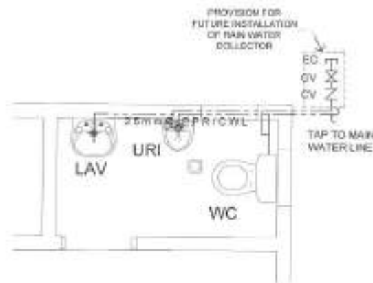
4 GROUND FLOOR C.R. WATERLINE LAYOUT ( PUMAREN BUILDING )
