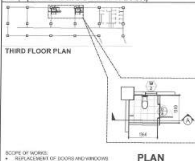
2 TYPICAL CLASSROOM TOILET LAYOUT (SB BUILDING-SECOND FLOOR)
